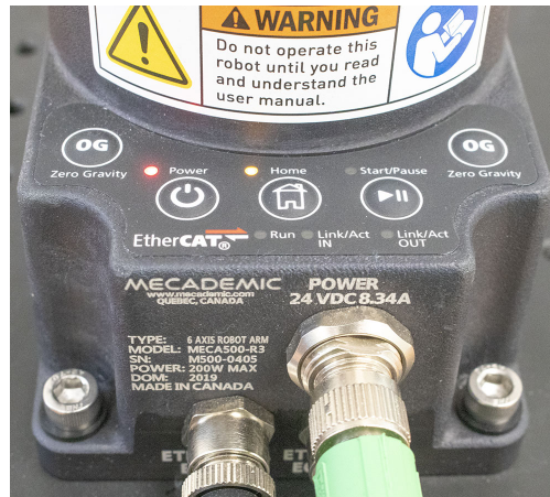
Figure 15: Robot control panel
