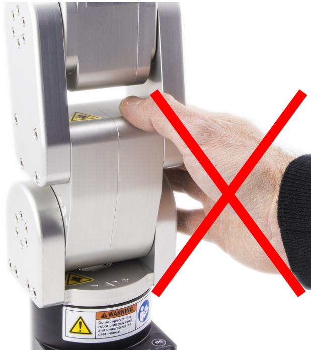
Figure 2: When the Meca500 is activated, keep away from the zones labeled with the pinch-point warning sign, to avoid injuries.
